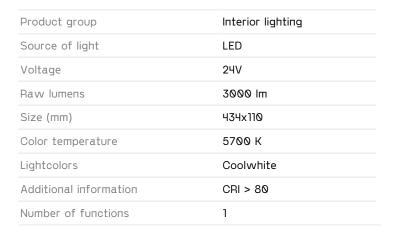
Manufacturer: Frensch Assembly: Surface Model: F-110 Shape: Rectangular Power: 28W Switch: No
